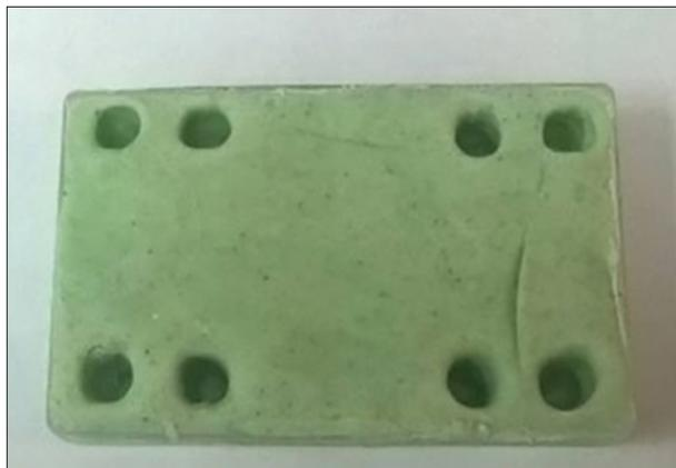
**Figure 1:** A rectangular acrylic block with eight holes in each block to support the teeth
